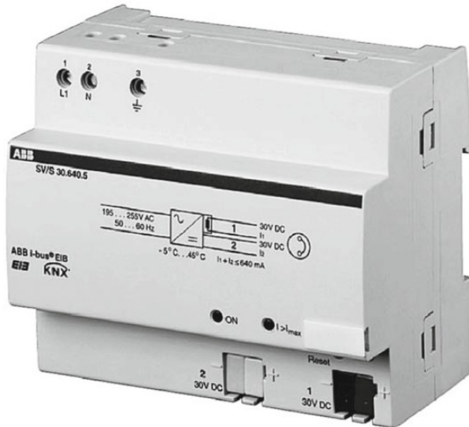
Fig. 3.13 A power supply unit 640 mA (RM) with an integrated choke and two 30 V DC outputs [ABB06]
