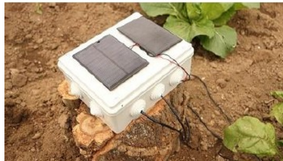
LoRa Long Range Sensor Monitoring – Reporting Sensor Readings from Outside: Soil Moisture and Temperature
