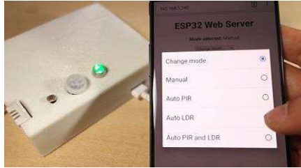
ESP32 Wi-Fi Multisensor – Temperature, Humidity, Motion, Luminosity, and Relay Control
