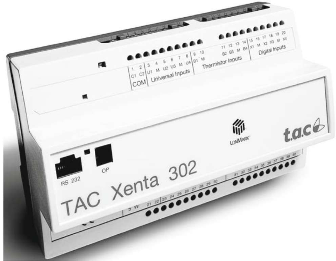
Fig. 1.2 A direct digital controller (DDC) [TAC02]
