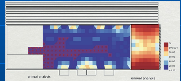
Useful daylight illuminance (UDI) map above 2000 lux for the Coworking and balcony area
