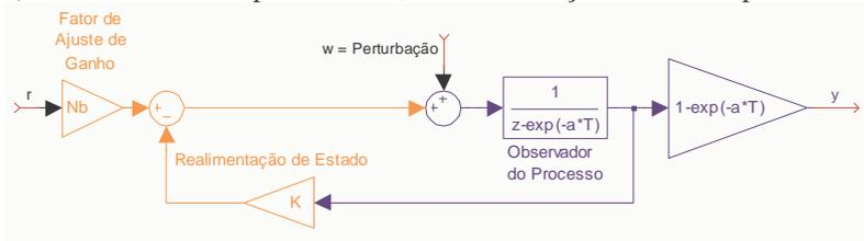
$$T = 0,5; \quad \frac{Y(z)}{R(z)} = Nb \frac{1 - \exp(-0,25)}{z - \exp(-0,25) + K} = \frac{Nb b}{z - c + K}$$
