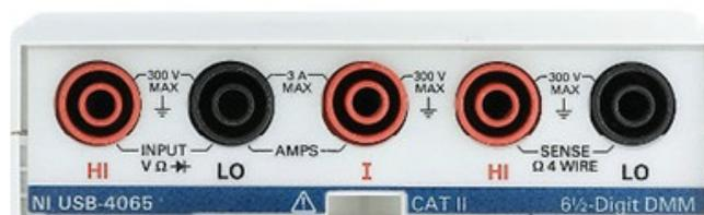
Figura 5.11: Multímetro digital NI USB-4065 DMM [19].
