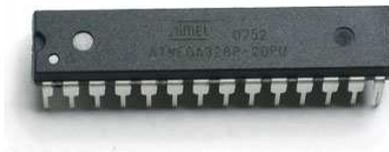
Figura 3.17. Microprocessador ATMEL, ATMEGA328p.
