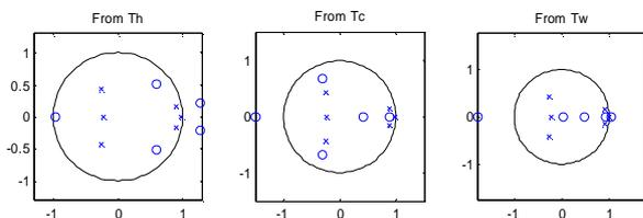
Figure 7. Three pole-zero maps of the 5 inputs MISO.
