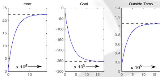
Figure 5. Step responses of a 3 inputs, 6<sup>th</sup> order linear MISO.
