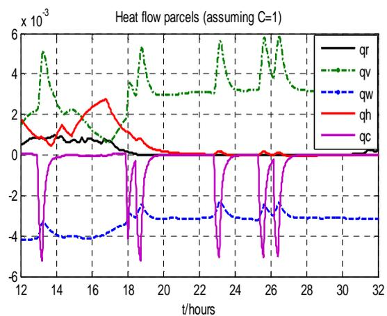
Figure 11. Heat flow obtained with the first-principles structured identification.
