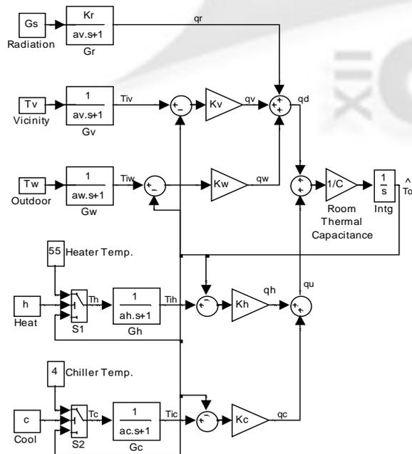
Figure 10 First-principles structured thermal model.
