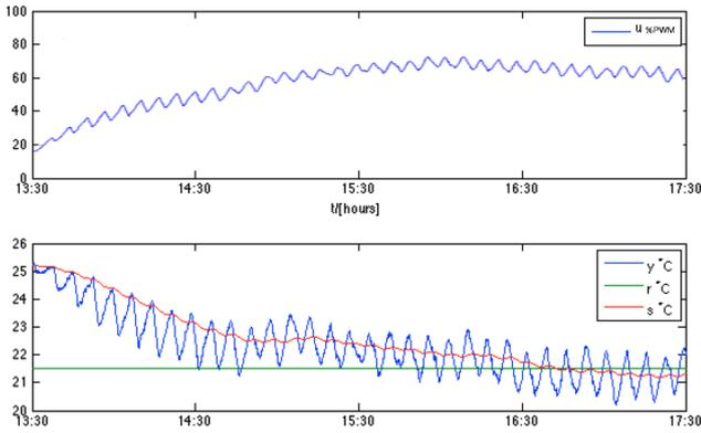
Fig. 11. Typical results for PI control. Experiment with variable thermal load.
