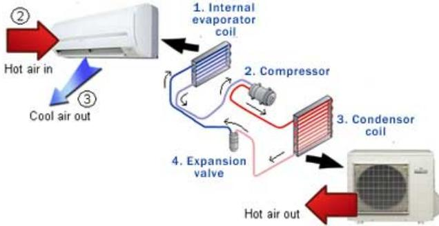
Fig. 3. Split air conditioner. (adapted airintelligence.co)
