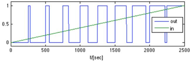
Fig. 4. Modified PWM for air conditioners,  $T_{cicle} = 250sec$ .
