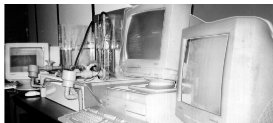
Fig. 6. Remote level control experiment: The three computers involved. From left to right: client, process controller and Web server. In this case the client is in the laboratory, but accessing the experiment like would any other Internet connected user.
