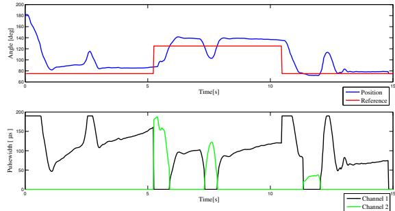
Figure 6: Subject 2. Elbow joint control and the effects of disturbances. A disturbance inducing positive displacement was applied at  $t = 2, 5\text{ s}$  and  $t = 12\text{ s}$ , while another disturbance producing negative displacement was applied at  $t = 7\text{ s}$ . Biceps bracchi activation level is pictured in black and Triceps bracchi in green.
