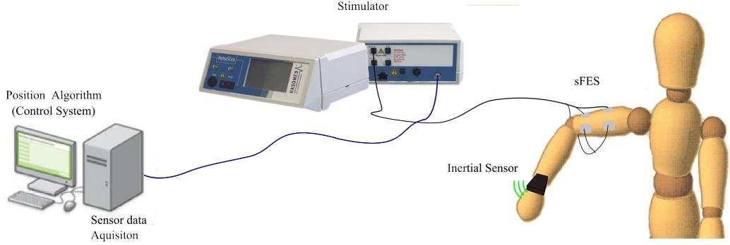
Figure 1: Closed-loop FES system for controlling elbow motion. Both stimulator and inertial sensor communicate with a PC, in which the proposed controller is implemented.
