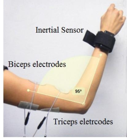
Figure 2: Photograph representing placement of sensor and electrodes, as well as the representation of the standard used for angle displacement (in light color).
