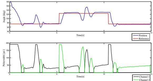
Figure 5: Subject 1. Elbow joint control and the effects of disturbances. A disturbance inducing positive displacement was applied at  $t = 2, 5\text{ s}$ , while another disturbance producing negative displacement was applied at  $t = 7\text{ s}$ . Biceps bracchi activation level is pictured in black and Triceps bracchi in green.
