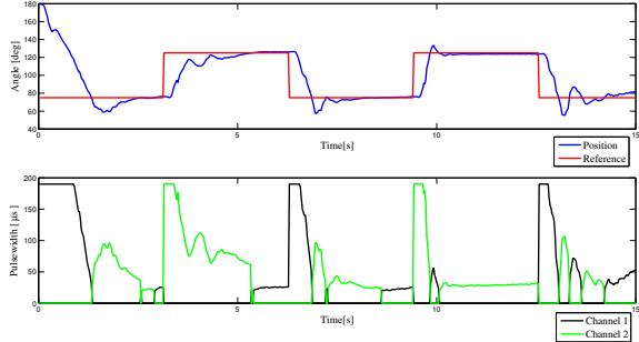
Figure 3: Subject 1. Elbow joint control without any disturbance. Biceps bracchi activation level is pictured in black and Triceps bracchi in green.
