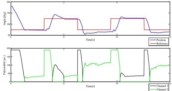
Figure 4: Subject 2. Elbow joint control without any disturbance. Biceps bracchi activation level is pictured in black and Triceps bracchi in green.
