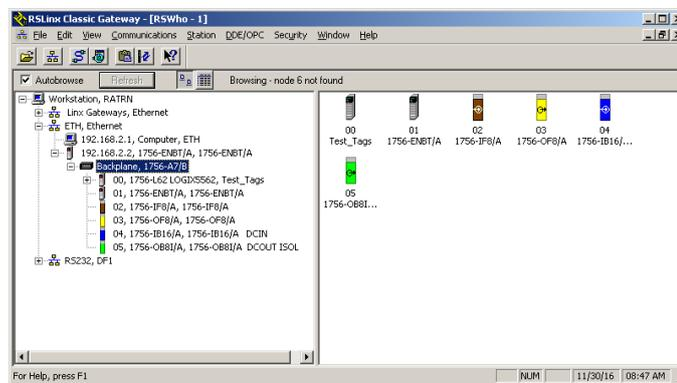
Figure 2.6: Interface do Software RSLinx.
