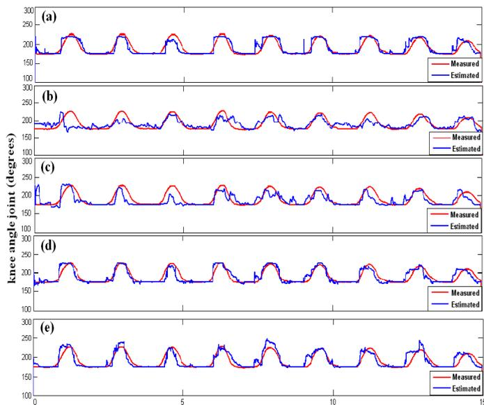
Fig. 6: Measured and estimated knee angle displacements: (a) algorithm from ref. [6]; (b) algorithm from ref. [17]; (c) algorithm from ref. [11]; (d) first algorithm based in data fusion; (e) second algorithm based in data fusion.
