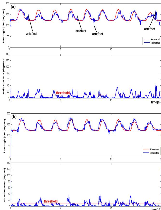
Fig. 5: Measured and estimated knee angle displacements and their absolute difference (estimation error): (a) first strategy; (b) second strategy. The threshold level used for calculating the statistics of the error events ( $10^\circ$ ) is indicated.
