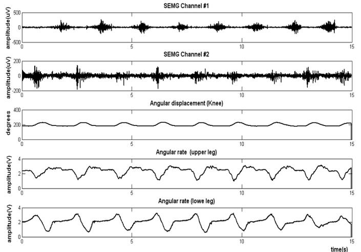
Fig. 4: Representative set of simultaneously-acquired SEMG signals (rectus femoris and semitendinosus muscles), electrogoniometer angle (knee), and gyroscope measurements (upper and lower legs).
