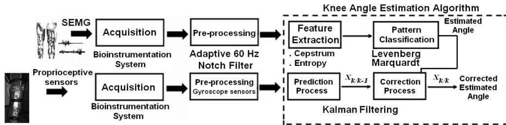
Fig. 2: Block diagram of the proposed knee angle estimation algorithm based on the second data fusion strategy.
