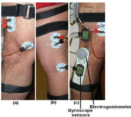
Fig. 3: Placement of SEMG electrodes (a,b), electrogoniometer and gyroscope sensors (c).
