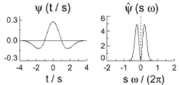
Figure 1 - Wavelet DOG with  $m = 2$ ; left, time domain; right, frequency domain.
