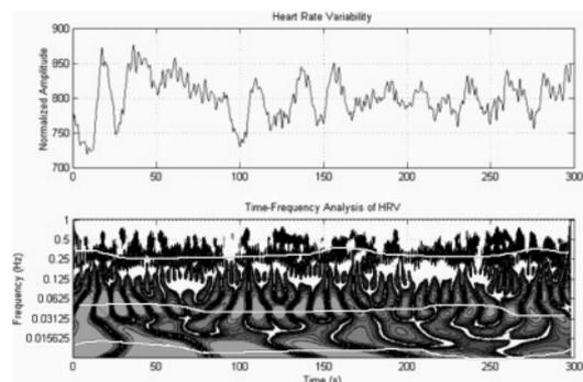
Figure 2 – HRV of normal segment of ECG; top, time domain; bottom, time-scale domain with lines marking the trajectories of VLF, LF and HF spectral clusters.
