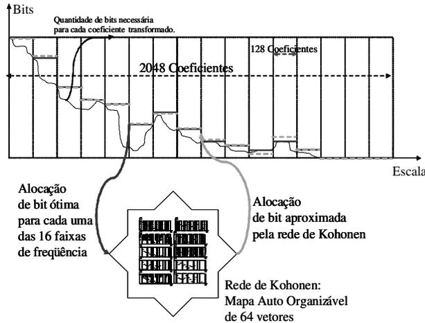
Fig. 3. - Illustration of the bit allocation algorithm.
