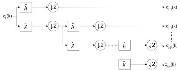
Fig. 1. Wavelet Decomposition Algorithm.
