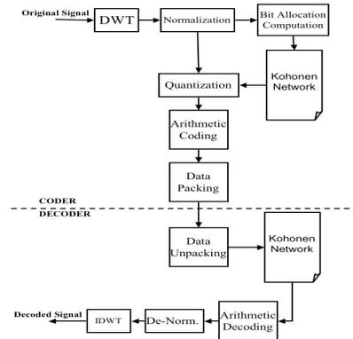
Fig. 2. Block-diagram of the proposed encoder and decoder.
