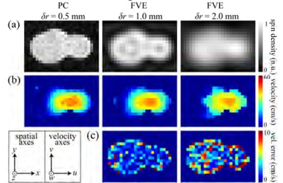
**Figure 1:** (a) Spin-density maps for PC (0.5 mm spatial resolution), FVE with 1 mm spatial resolution, and FVE with 2 mm spatial resolution, for a slice perpendicular to a carotid phantom's bifurcation; (b) corresponding velocity maps; and (c) absolute error for the FVE-estimated velocity maps, relative to the PC reference.
