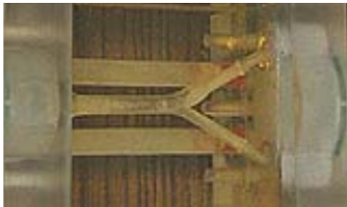
Figure 1. Carotid flow phantom (Phantoms by Design, Inc., Bothell, WA).
