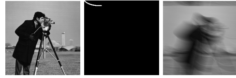
Fig. 6. Motion blur. (a) Ideal image f . (b) Trajectory mask h_{motion} , expressing the relative motion of the camera with respect to the scene objects. (c) Image containing motion blur: g = f \otimes h_{motion} .
