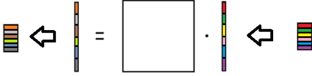
Fig. 4. Representing a 2D image with R rows and C columns as a 1D vector containing R \times C elements (right), which can then be transformed using a matrix-vector multiplication (center). The transformed vector is then decoded back into an image with R rows and C columns.
