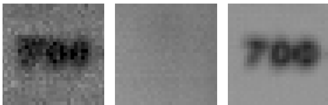
Figure 12: Noise analysis. The left image is a close-up of a conventional photo at f/22 , the middle is a conventional photo at f/4 (completely blurred due to misfocus), and the right image is a refocused light field photograph shot at f/4 . All exposure durations were the same (1/60 sec), and the left image has been scaled to match the brightness of the other two. The light field photo (right) is much sharper than the conventional one at the same aperture size (middle). It is as sharp as the conventional f/22 photo, but its SNR is 5.8 times higher.
