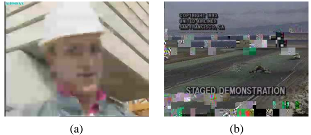
Fig. 1. Sample video frames containing medium and severe intensity packet-loss impairments.
