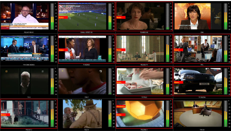
Fig. 8 Example of screens of NET-MOZAIC showing the alarms. Alarms are displayed as color (yellow or red) frames around the channel window. The name of the metric causing the alarm appears as text on the red or yellow bar
