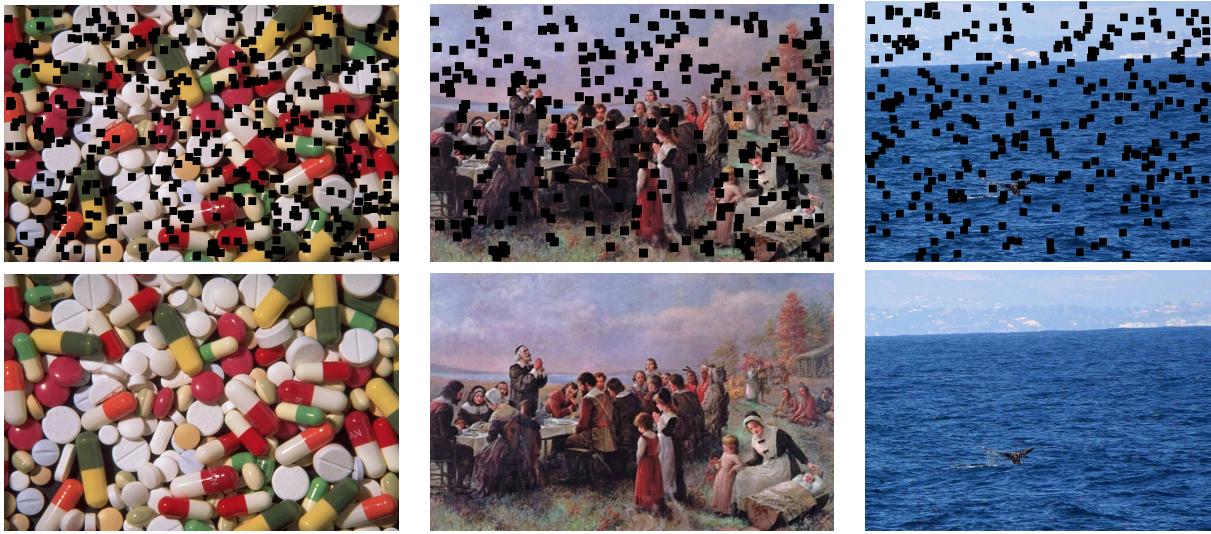
Fig. 7. Illustration of restoration of lost blocks using proposed error concealment algorithm: (top) pictures with 20% of content lost and (bottom) restored pictures using the proposed algorithm.
