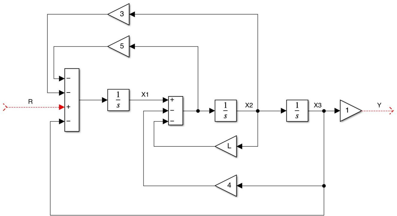
$$\frac{Y(s)}{R(s)} = \frac{P_1}{Delta}; \quad P_1 = \frac{1}{s^3}; \quad Delta = 1 + \frac{5}{s} + \frac{L}{s} + \frac{4}{s^2} + \frac{3}{s^2} + \frac{1}{s^3}; \quad \frac{Y(s)}{R(s)} = \frac{\frac{1}{s^3}}{1 + \frac{5+L}{s} + \frac{7}{s^2} + \frac{1}{s^3}} = \frac{1}{s^3 + (5+L)s^2 + 7s + 1}$$
