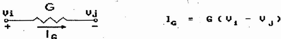
Fig. 2.1 - Resistor Linear
